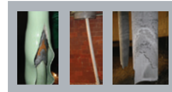
Fig. 9: Common dilution water dip pipes. PTFE encapsulated carbon steel (left), solid PTFE tube (middle), and Alloy (right).
